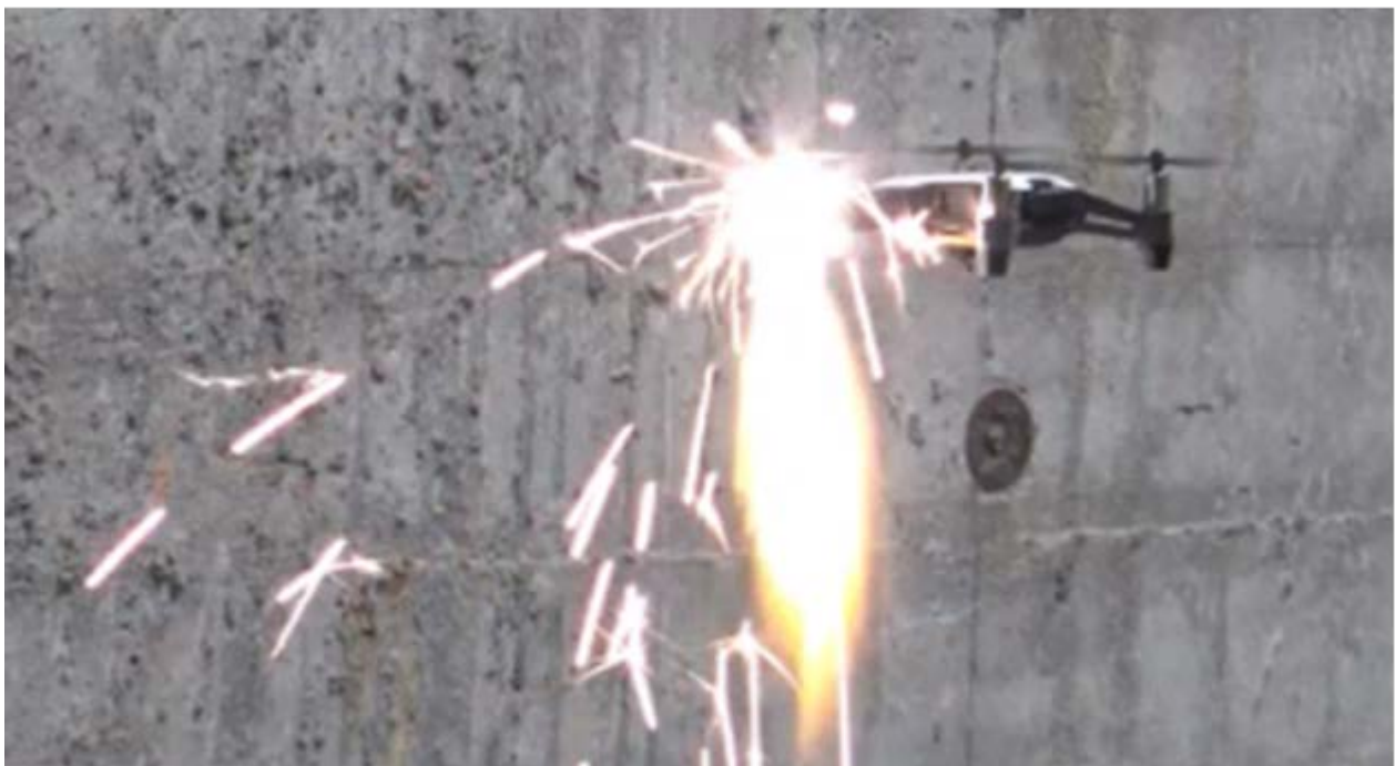
Figure 5: Laser engagement of a DJI Tello drone.
